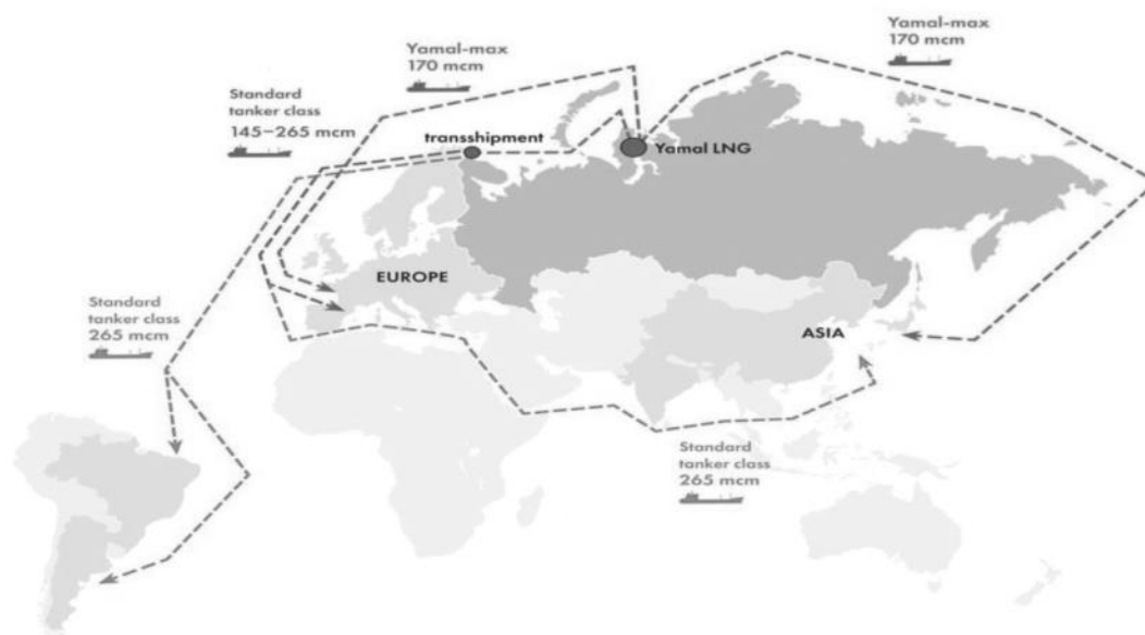
Figure 7 - Routes for LNG transportation options via NSR and the Suez Canal [Mazneva, www]
