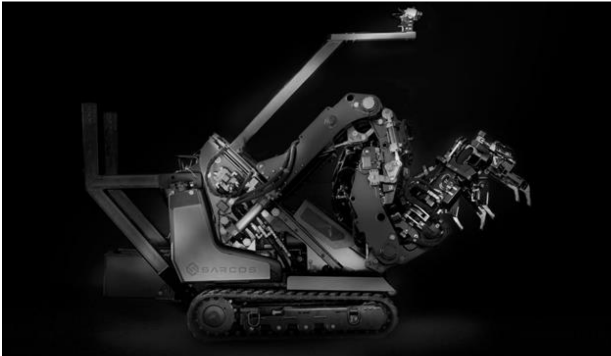
Figure 5 – Guardian XO by Sarcos Robotics. Gain 20 times: when lifting 90kg in the hands of an exoskeleton-4.5 kg in the hands of a person. For sale: 2020
